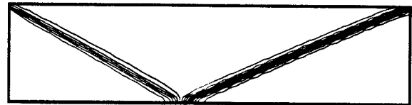
Figure 2. Pressure contours, M_\infty = 2.9 .
