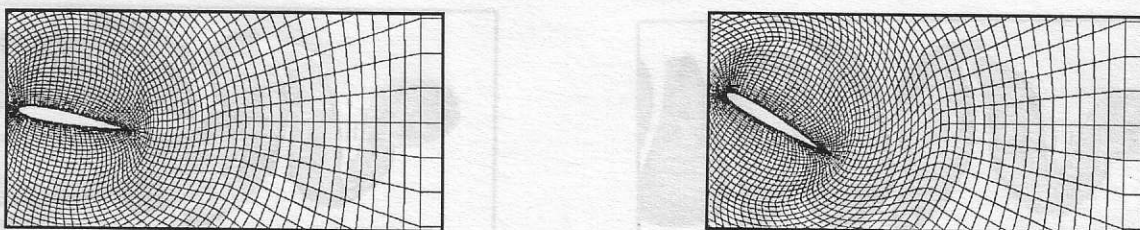
Figure 7. Flow past an oscillating NACA 0012 airfoil at Reynolds number 1,000: mesh at 10° and 30° angle of attack.
