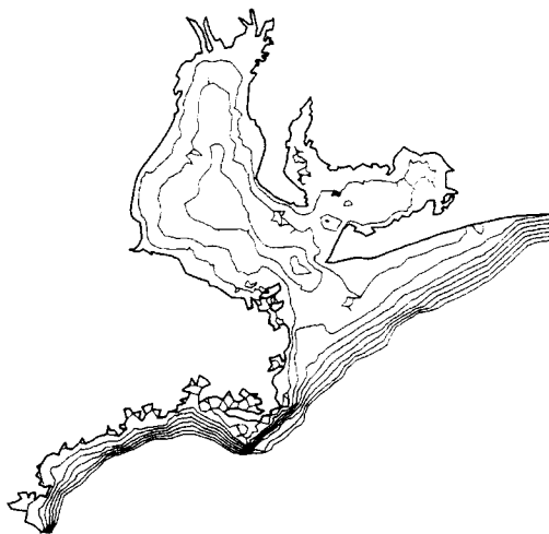
Figure 7. Water depth diagram around Ise-Bay (contours are evenly spaced at 10 m intervals)
