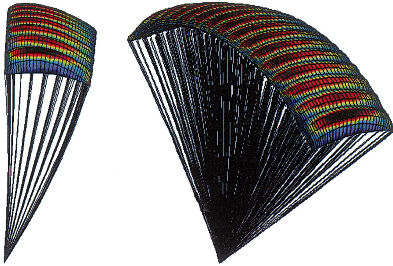
Fig. 9. FSI simulation: maximum principal stress distribution on the canopy surface. Red indicates high stress, while blue indicates low stress.
